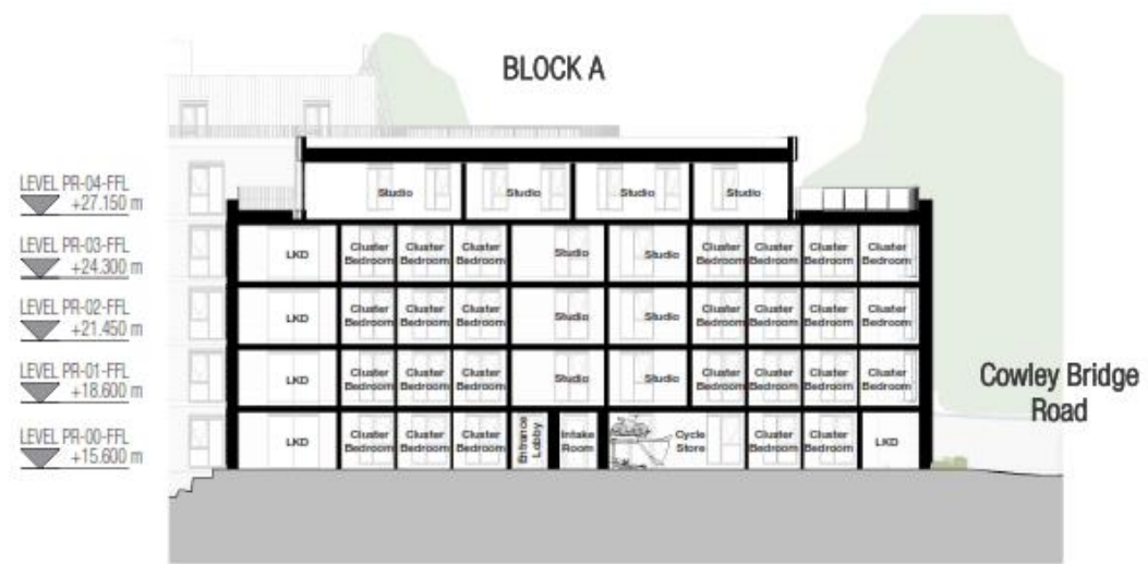
SITE SECTION A (Through Block A)
