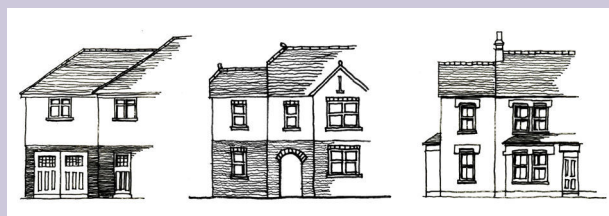
Figure 1.5 Extensions should reflect the character and appearance of the main house in terms of scale, roof form, materials and architectural details such as windows and doors.
