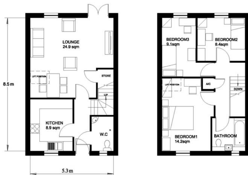
Figure 9.7 An example of a 3 bedroom house which meets the standards. Gross internal floor area 90 square metres
