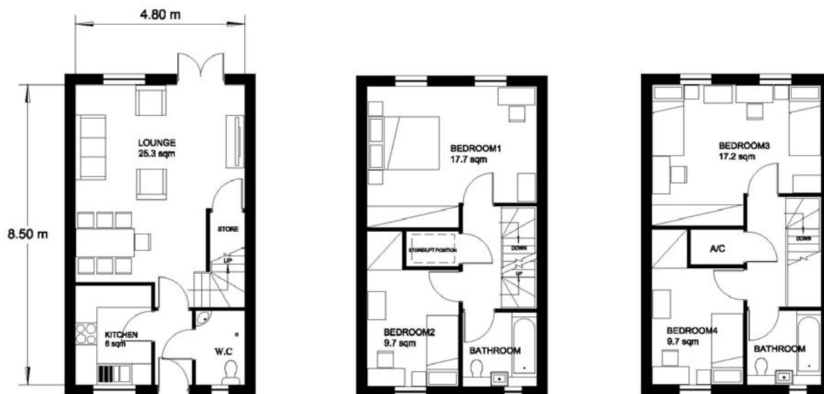
Figure 9.10 An example of 4 bedroom townhouse which meets the standards, Gross Internal Floor Area 117.6 sq metres.
