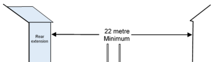
Figure 4.4: Back-to back distances: a minimum of 22 metres between the rear walls of the properties should be achieved in the interest of privacy and minimising overlooking.
