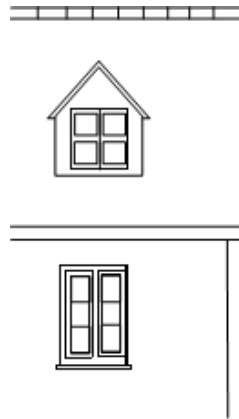
Figure 6.2: The dormer's size allows the main roof to remain the dominant feature, and the dormer window is smaller than the window on the floor below.
