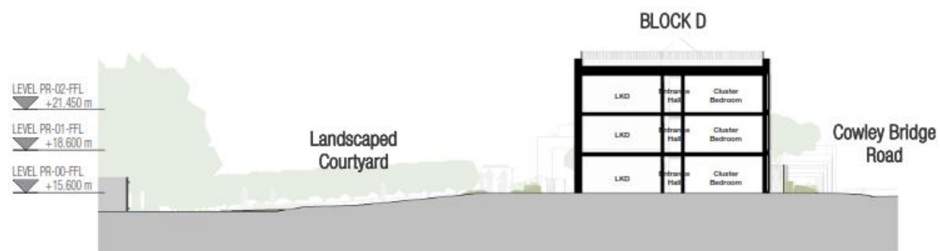
SITE SECTION E (Through Block D)
