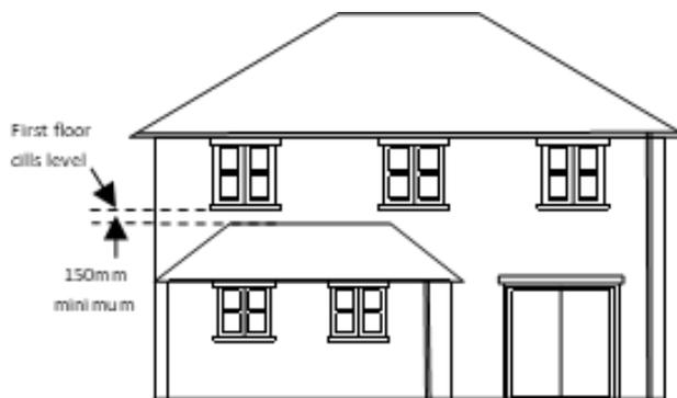
*Figure 4.7: Single-storey extension with 150mm gap between extension ridge and windowsills of the first-floor windows.*
